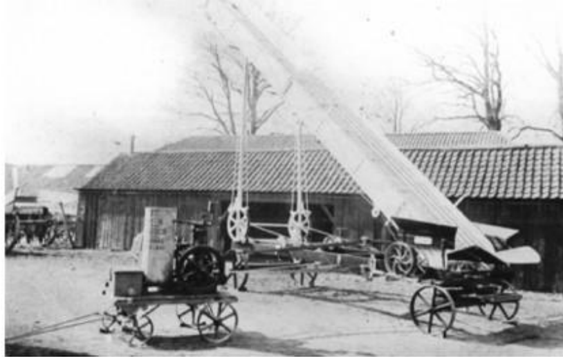
Reeves 'Advance' elevator, with troughs raised. Chains are driven by a Fairbanks Morse portable oil engine, through belt drives. The two-storey building in the distance houses the carpenters' shop (ground floor) and tinsmiths' shop above. Circa 1912
